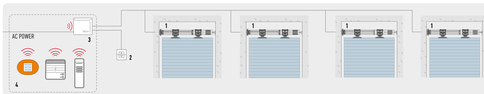
1. TUBULAR MOTOR 2. GENERAL "UP/DOWN" BUTTON 3. TT4 SERIES CONTROL UNIT 4. TRANSMITTER FOR GROUP CONTROL
