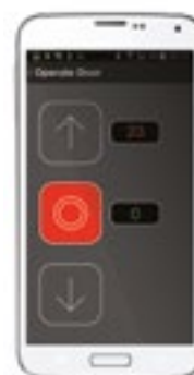
APP FOR CONTROL UNIT PROGRAMMING BY ANDROID SMARTPHONE OR TABLET THROUGH BLUETOOTH CONNECTION.
