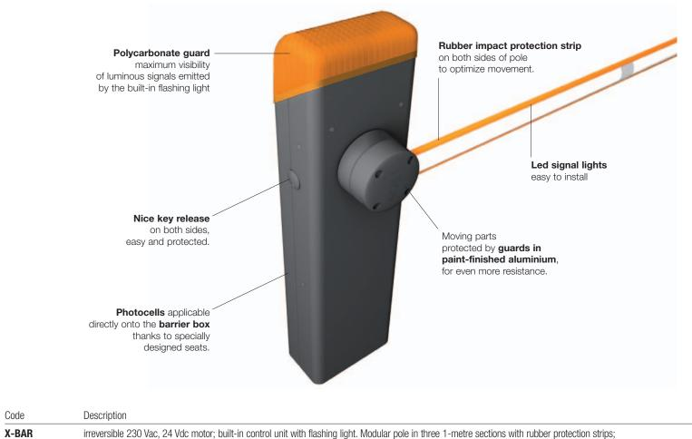
enclosure in galvanized and paint-finished steel. Nice BlueBUS technology and compatibility with the systems Nice Opera and Solemyo.
