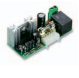
CARICA plug-in card for battery charger Pc./pack 1
